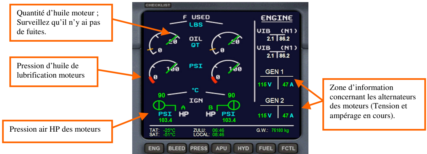
Image 22 – ECAM2 Page Engines
