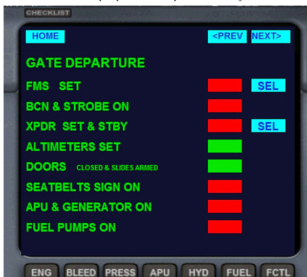
Image 21 – ECAM2 Page Gate Departure de la Checklist
