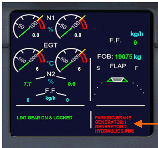
Picture 19 – Primary upper ECAM when avionics is powered
