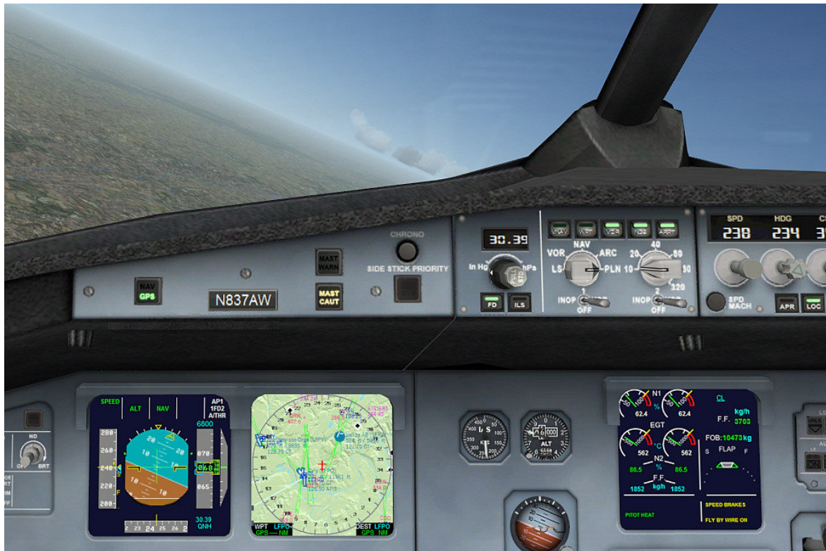
Picture 16 – ND Radar map terrain with the PLN position
