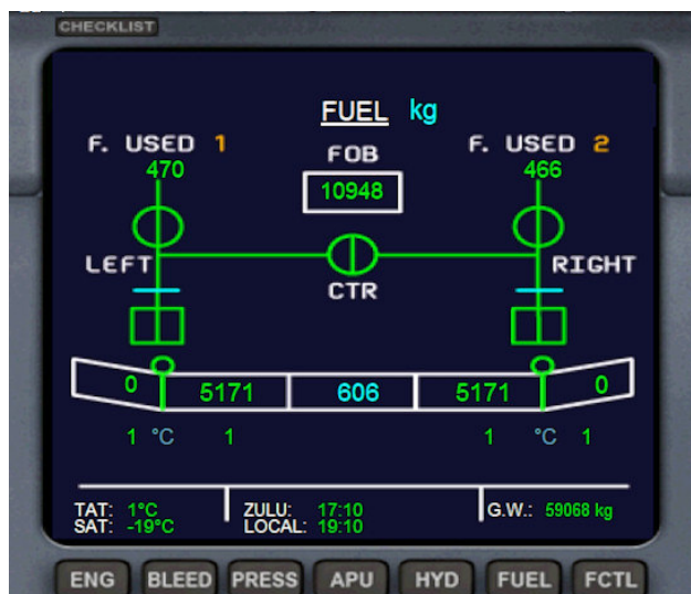
picture 36 – Engines fed by wings tanks now
