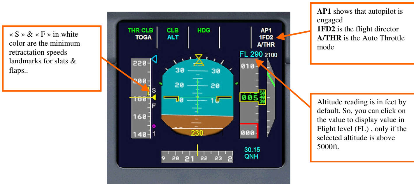
Picture 2 PFD at takeoff with VNAV mode and AutoThrottle
