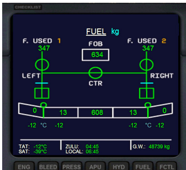
Picture 41 – opening of the CROSSFEED in case of low fuel level
