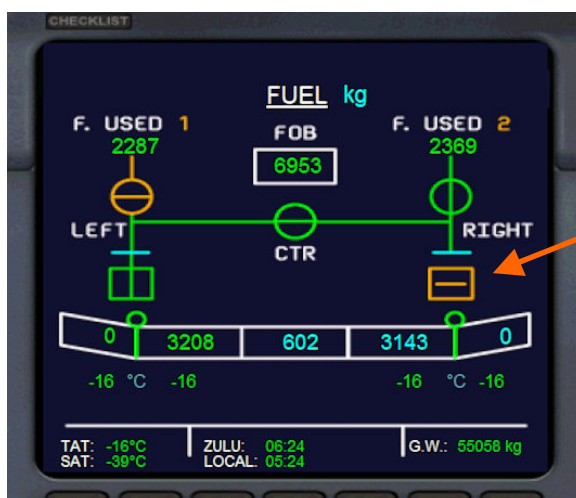
Picture 39 – CROSSFEED left engine from right wing tanks
