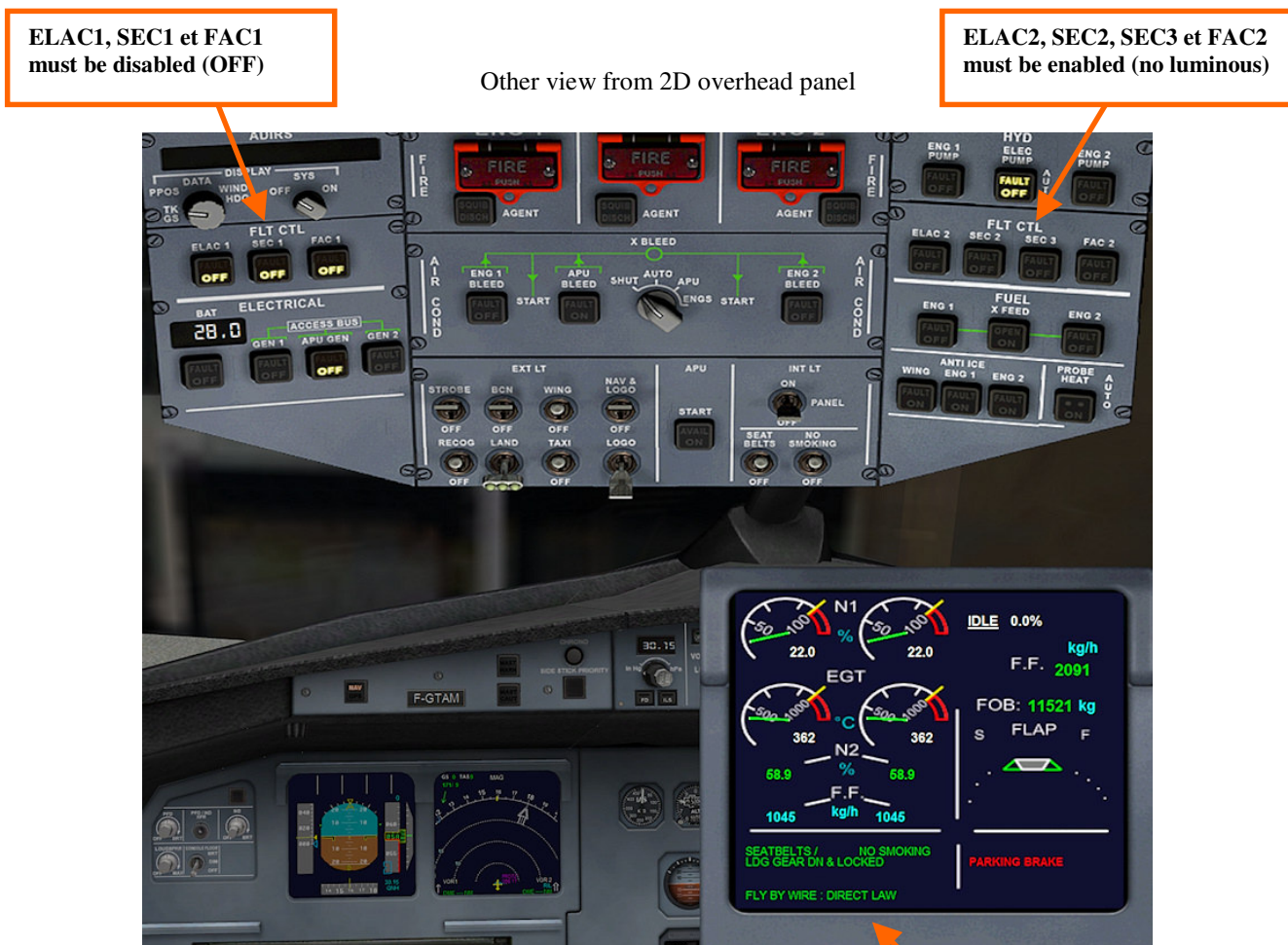
Picture 70 – FBW in DIRECT LAW mode – 2D overhead panel view with message on primary ECAM
