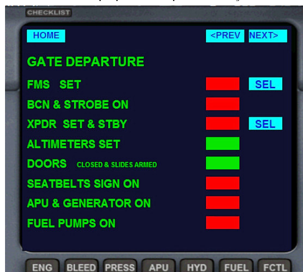
Image 21 – ECAM2 Page Gate Departure de la Checklist
