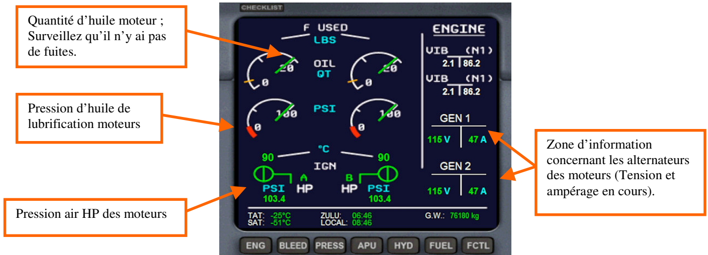
Image 22 – ECAM2 Page Engines
